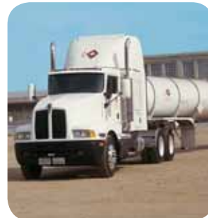
Kynar-lined vacuum tankers for transport of low pH acids
